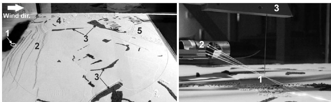
Figure 1: Left: Model of scale ratio 1:3300 positioned at wind-tunnel including point source of pollutant (1) integrated at the bottom of special inclination smoothly connected to east end of coal mine (2), necessary vegetation (3), south part of town Chomutov (4) and village Droužkovice (5). Right: simultaneous point (1) measurements of two velocity components and concentrations by LDA (2) and FFID (3), respectively, above the model during measurements
