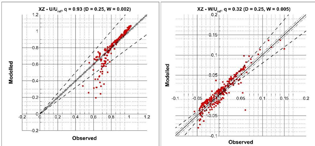
Figure 7: Scatter plots and *Hit Rates* for  $u/u_{ref}$  (left) and  $w/u_{ref}$  (right) at plane  $xz$ . Dashed lines represent  $D$  and dash-and-dot  $W$ . Red points that are within these lines are counted as hits ( $N_i = 1$ ).
