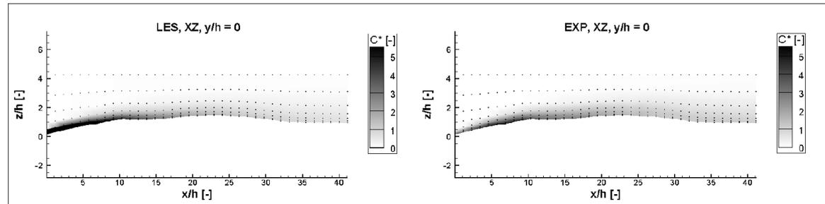
Figure 6: Comparison of LES (left) and wind-tunnel (right) mean dimensionless concentrations  $C^*$  at plane  $xz$  parallel with approach wind direction positioned at the point source origin ( $y/h = 0$ ).
