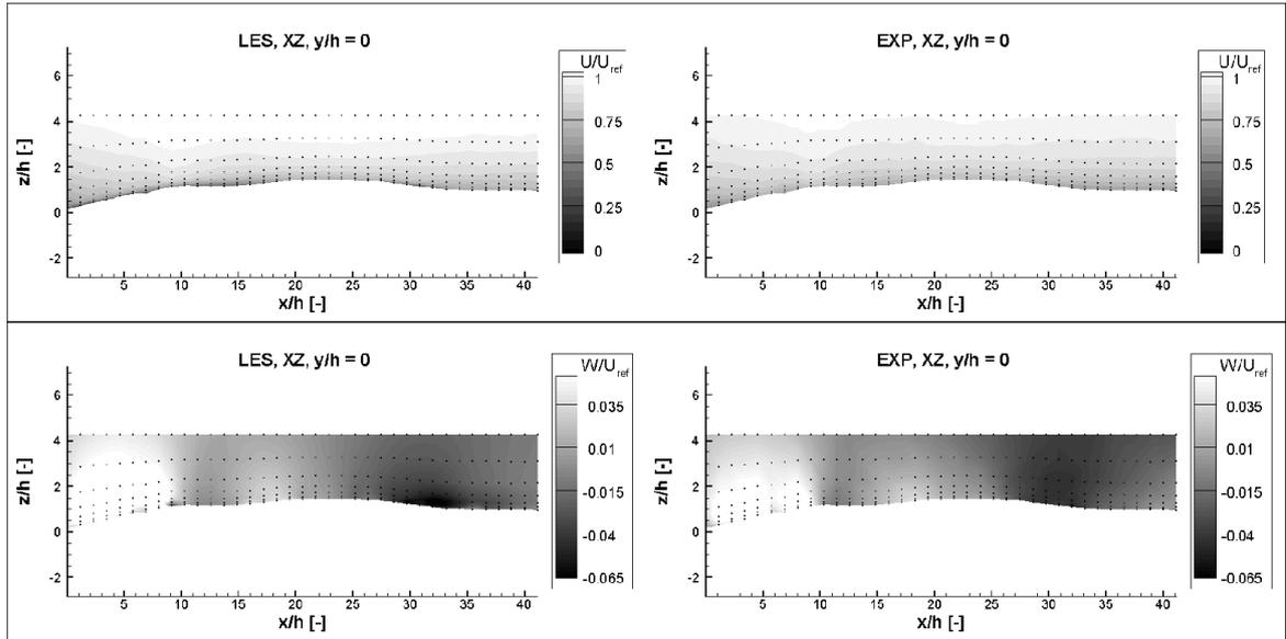
Figure 5: Comparison of LES (left) and wind-tunnel (right) mean dimensionless longitudinal  $u/u_{ref}$  (up) and vertical (down) velocities  $w/u_{ref}$  at plane  $xz$  parallel with approach wind direction positioned at the point source origin ( $y/h = 0$ ).
