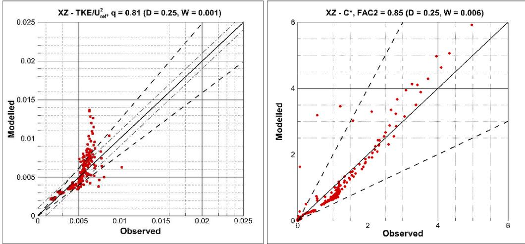
Figure 8: Scatter plots of  $TKE/u_{ref}^2$  (left) and  $C^*$  (right) at plane  $xz$ . Dashed lines represent fractional deviation  $D$  and dash-and-dot absolute deviation  $W$ . Red points that are within these lines are counted as hits ( $N_i = 1$ ). For  $C^*$  the  $FAC2$  metric was used.
