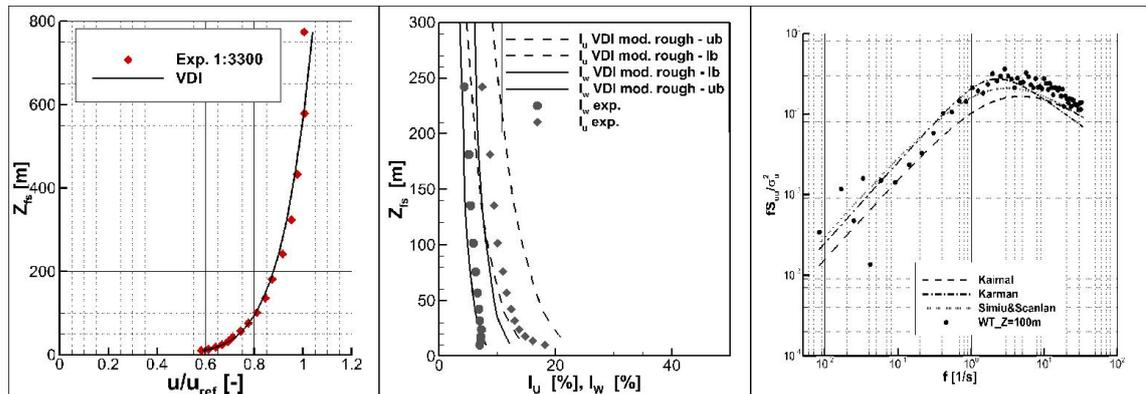
Figure 2: The vertical profile of dimensionless longitudinal velocity  $u/u_{ref}$  (left), vertical profiles of turbulence intensities  $I_u$ ,  $I_w$  (middle) and longitudinal velocity turbulence spectrum  $S_{uu}$  of modelled boundary layer at full scale height 100m above the terrain ( $WT\_Z=100$ ) compared with Kaimal, Karman and Simiu&Scanlan spectra (right).
