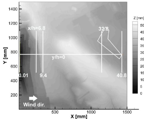
Figure 4: Measured 5 vertical planes  $yz$  (vertical lines –  $x/h$ ) and one vertical plane  $xz$  (horizontal line –  $y/h$ ) displayed on model contour map. Approach wind direction is from left to right. Note the elongated hill in the middle of the model (white contours) and coal mine escarpments (the most left in the picture).
