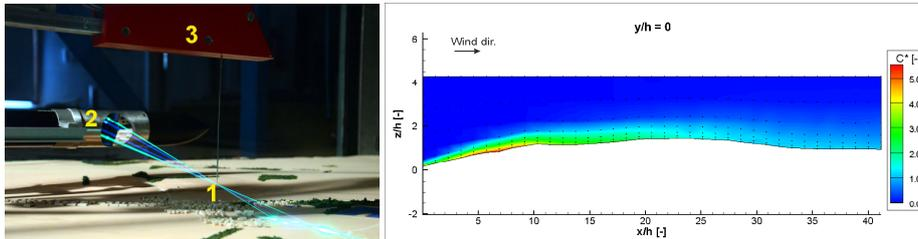
Fig.1 Left: simultaneous point (1) measurement of two velocity components and concentrations by LDA (2) and FFID (3), respectively, during the wind-tunnel experiment; Right: dimensionless concentrations measured at vertical plane parallel to wind direction.
