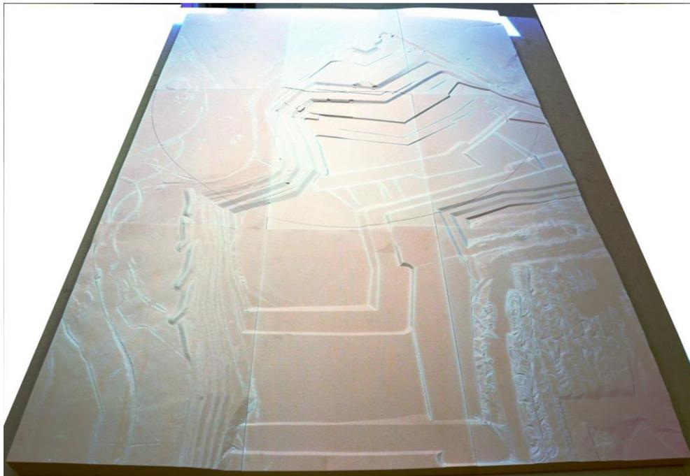
Figure 5. Aerodynamic research: a model for visualization of flow fields in the wind tunnel by two-dimensional optical fibre Laser Doppler Anemometry.
